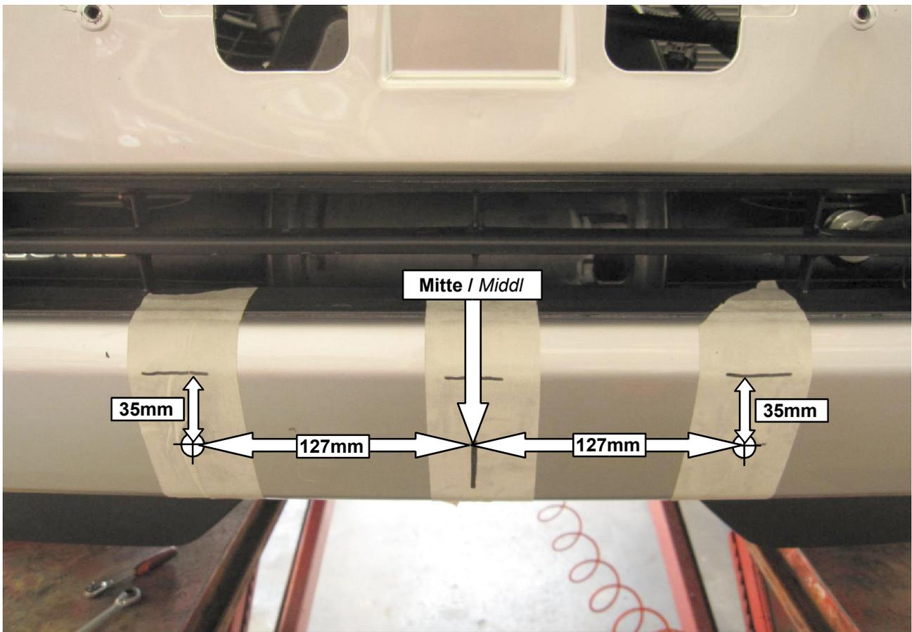
**21** Bohren  $\varnothing$  10,5mm / drill  $\varnothing$  10,5mm
